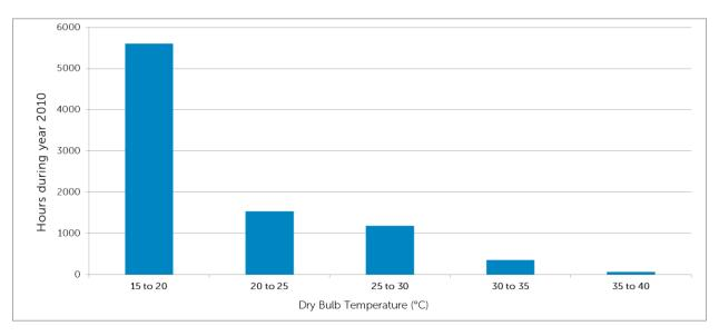
Figure 4. Inlet Temperatures of Chiller-less Data Center: New York City, 2010
