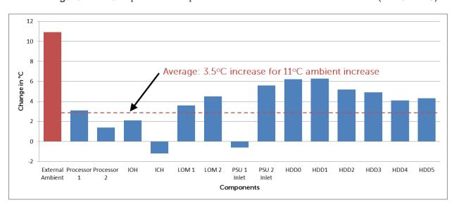
Figure 2. Component Temperature Increase Relative to Ambient (24°C-35°C)
