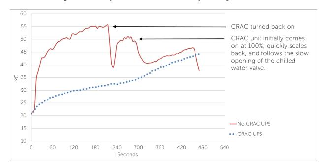
Figure 1. Temperature Rise After Facility Cooling Failure
